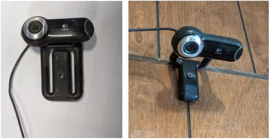
Left: Because it is made to mount on the top edge of a laptop, provisions need to be made to mount it to a wall for use as a puppy cam. Thus the drilled hole in the middle of the mount for a wood screw. Right: Mounted eight feet off the floor, this camera can view a 6x8 floor area
